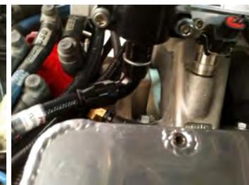
Disconnect the factory fuel line and remove it. The teflon feed line should route in the same direction and go under the throttle body to the fuel rail.
