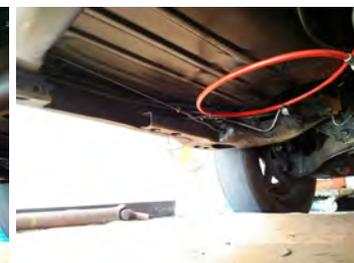
Step 3) Run each line up in the corner of the frame near the front, keeping it close to the edge of the frame and the floor board. In the engine compartment you will follow the same procedure keeping the lines closest to the plastic inner fender as you come upward on the right side of the steering arm.
