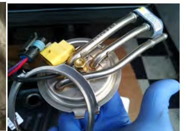
Step 3) This is how the sending unit looks like with the float on. The best way to get the float on the pump is to insert the pump in the tank and hold on to it. With a needle nose pliers, grab the side of the float and attach it to the pump inside the tank, then put the locking tab around the hanger of the float and secure the double pumper in the tank with the locking ring.
