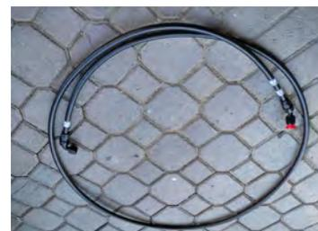
Step 4) Take out the feed line that connects the fuel rail, and the return line that connects to the fuel pressure regulator. because the are going to run in the same line together.
