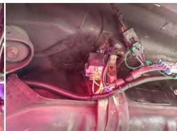
Follow the harness along the frame wedged inbetween the spring perch. At the top of the body of the car there is a opening where you can run the harness that will follow the contour of the fuel lines
