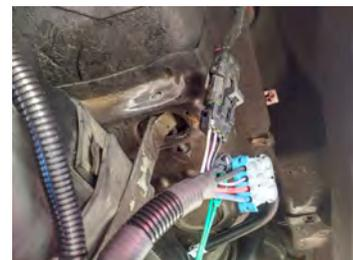
Step 4) Now lets secure the 2 relays. On the tank tank strap, there is a nut and bolt holding it to the body of the car. On the passenger side. take off the nut and mount the relay over the bolt and fasten it. Over on the driver's side. Do you same, but this time clean that area to bare metal and use the silicone lube supplied with the kit and apply a little to that area, then mount the relay and secure it with the nut.
