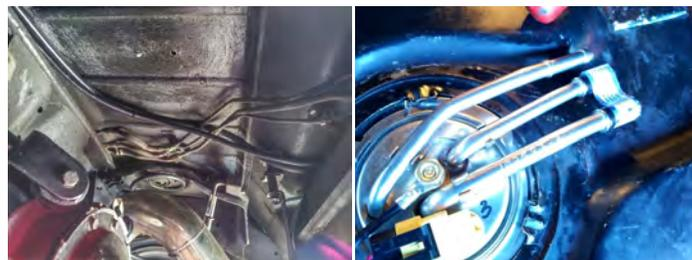
Step 4) Now you can attached both feed and return lines to the tank. In the first picture you see the end of the fitting. Unscrew the end, because that is what is going to tie in these lines
