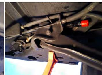
Then grab the end of that line and continue to run it upward to the top of the frame where it will exit the top area by the spring perch.
