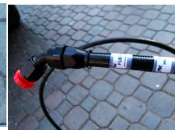
Run both lines along the frame where the factory fuel line is. Do not secure any of the lines with zip ties as yet.
