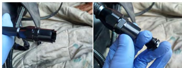
You will notice the open side of the end. Place the end over the lines on the double pumper feed and return. The end of the line on the sending unit has a ridge on it that will butt the fitting to it, securing the line. Place the line over the end of the fuel sending line and screw the end fitting back into the line the way it was originally, and tighten it up. Lastly, attach the rubber line from the factory for your vent on the sending unit and tighten it up.
